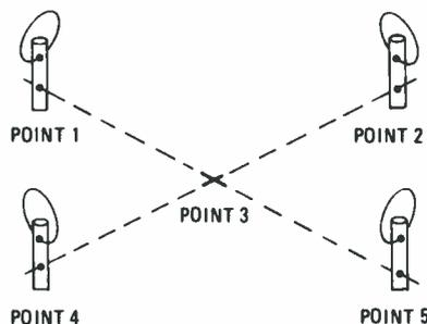
FIG. 2—TO PINPOINT a location, at least two readings should be taken. The point where the lines determined by those readings intersect is the general location of the transmitter. The more readings that are taken, the more precisely a location can be found.
